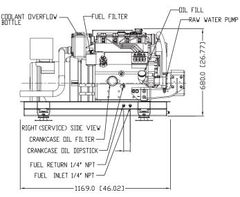
**M844LW3 Overall Dimensions L x W x H:** 46.0 x 22.8 x 27.5 inch (1169 x 580 x 697 mm) **Sound Enclosure Dimensions L x W x H:** 46.0 x 22.8 x 28.1 inch (1169 x 580 x 714 mm) **Sound Enclosure Weight:** 125.0 lbs. (57.0 kg)
