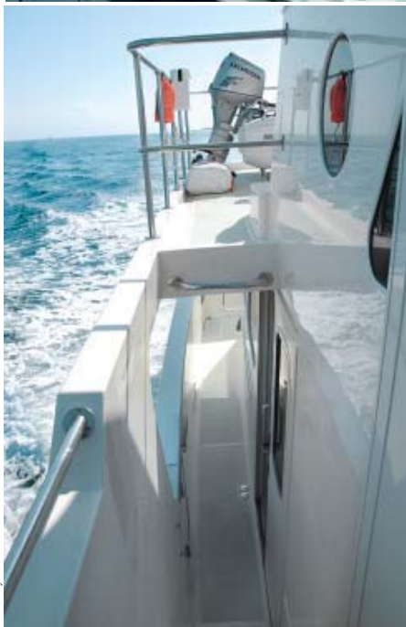
Top: With a single side deck, boarding and mooring are simplest on the Northwest 45's starboard side. The boat's asymmetrical design and a beam of 15 feet 10 inches create generous interior spaces. Above: The wide, covered side deck offers plenty of protection for the crew while under way.
